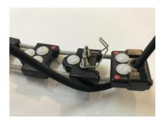
6) Screw a white plastic bolt on each grub screw
